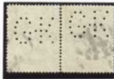
Die 2 Die 1 Punched in two operations
